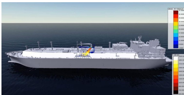
Fig. 2.6-2 Fire diffusion after jet leakage
