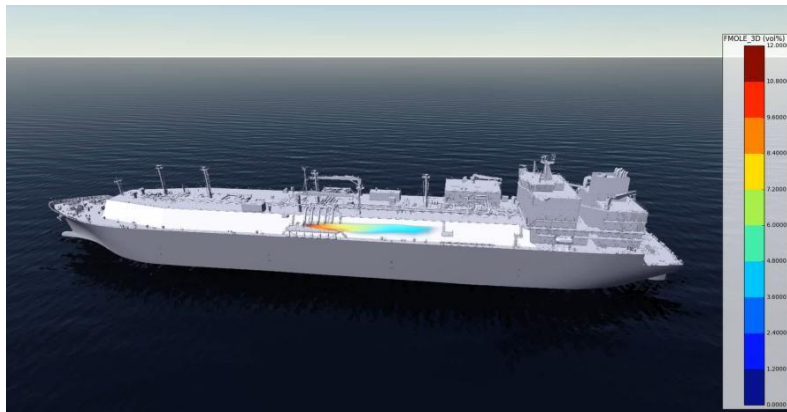
Fig. 2.6-1 Diffusion of vapor cloud after jet leakage
